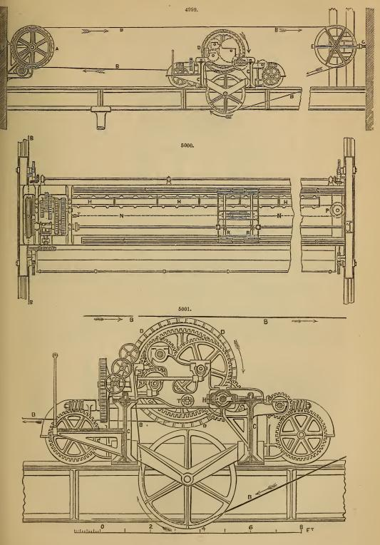
carrying pulleys to support it, and is consequently free from the friction that accompanies their use. The strop in which this crane works is 180 ft. long, and the rope hangs in a catenary curve
